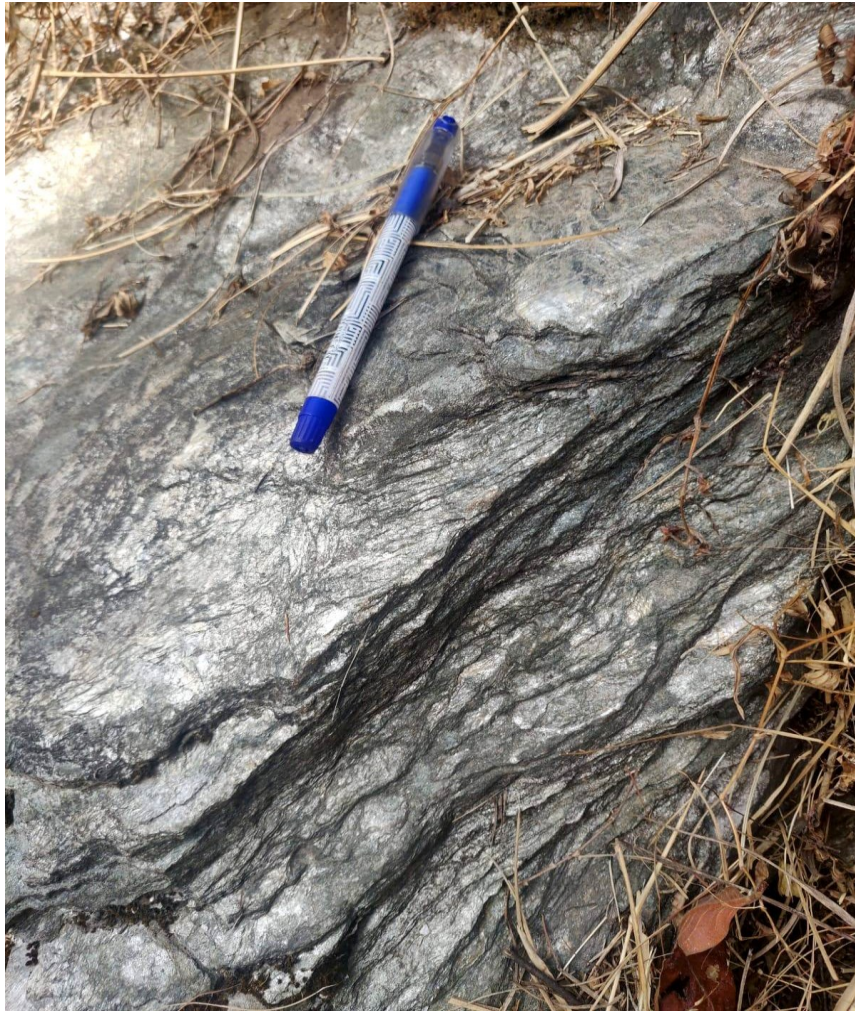
Plate – 4.1a Field photograph of Sericite Schist at Pelling, Gyalshing block, West Sikkim
